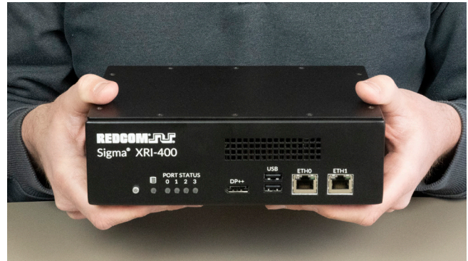
REDCOM Sigma® XRI-400 measures just 8.4 x 5.75 x 2.6 in and weighs 2.6 lbs.
