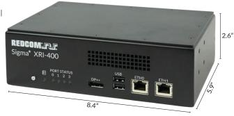
The small form factor of Sigma XRI-400 allows the solution to be mounted in aircraft, packed, hand-carried, or added to an existing data/comms rack to support all areas of operations.
